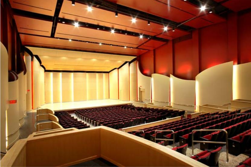
**FIGURE 2** Illustration of a hall with geometrical shaping to achieve acoustical diffusion
